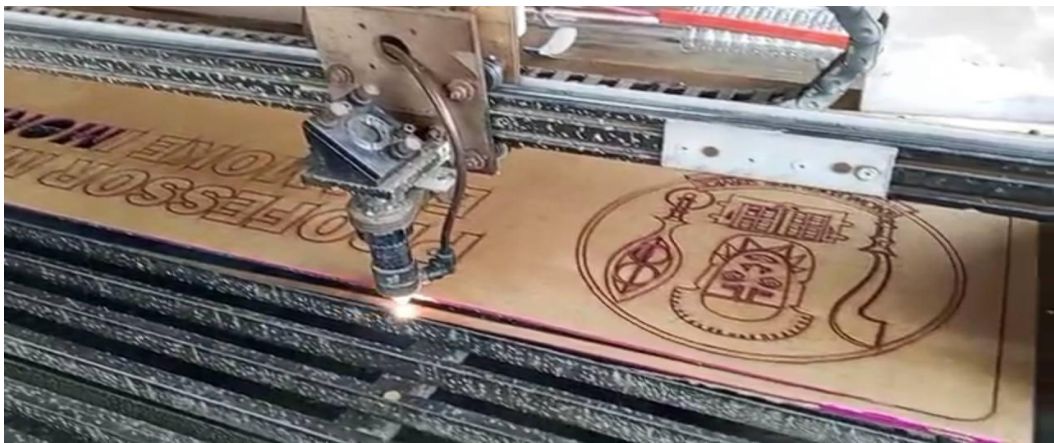
Fig: 6 Laser Cutting of the Acrylic Board
