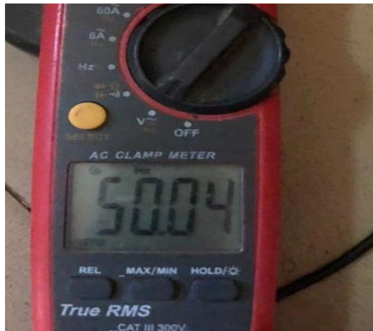
Figure 4.15: FREQUENCY OF OUTPUT VOLTAGE FOR LOCAL INVERTER
