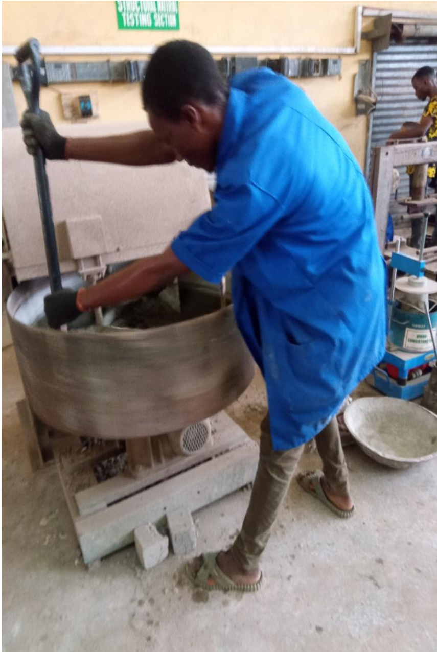
Mixing of concrete
