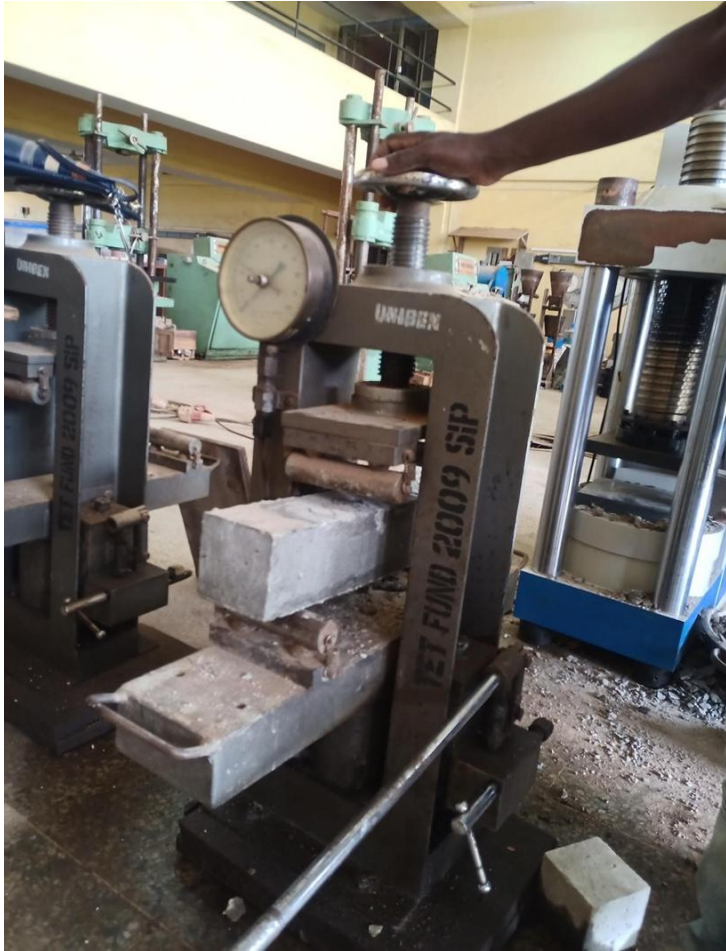
Flexural Test ongoing
