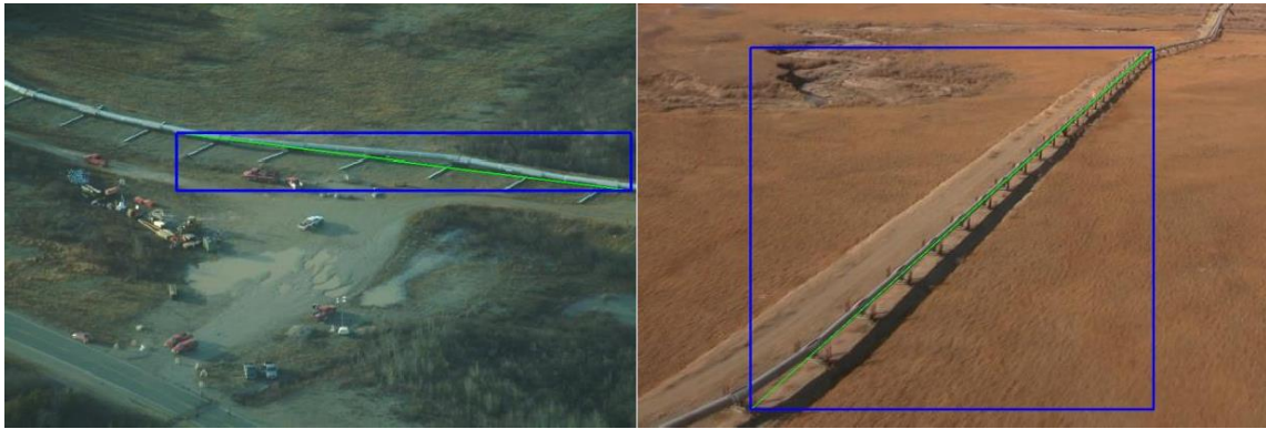
Figure 4-6: The longest line detection using Hough Transform
