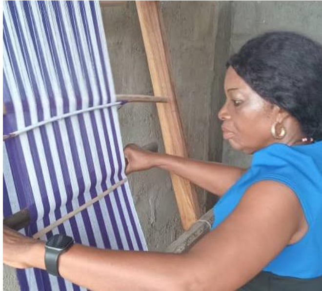
Pulling Down the Shed Stick to Create an Opening
