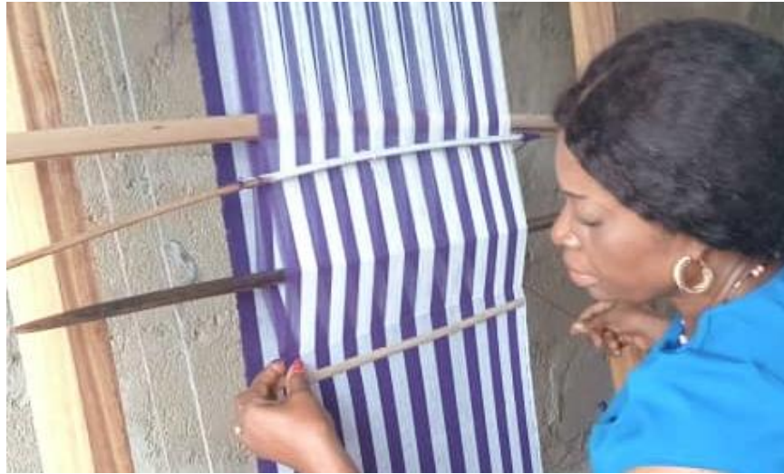
Controlling the Weft Yarn from Pulling Too Tight
