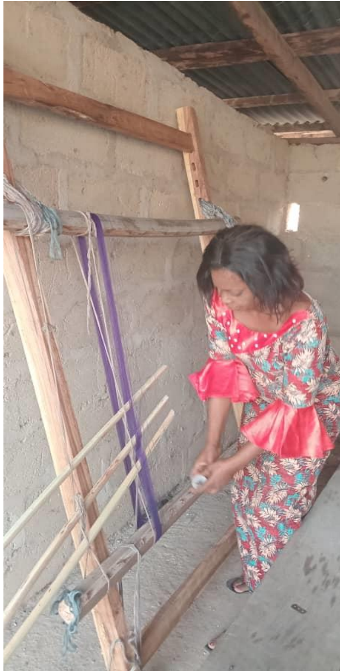
Warping the Desired Colour on the Loom
