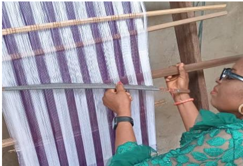
Pulling of the Heddle to Create Shed
