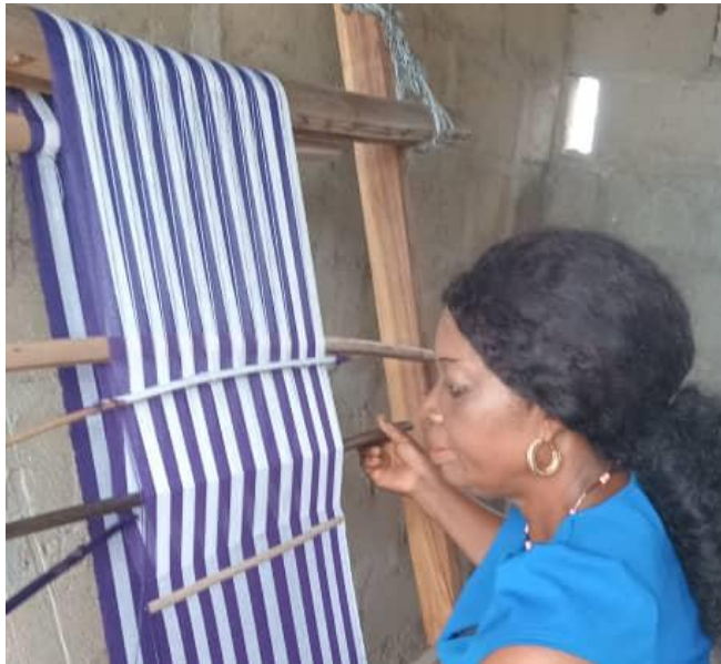
The Sword Being Inserted into the Opening Created by the Shed Stick
