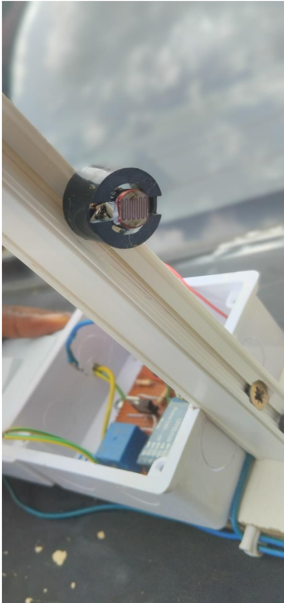
FIGURE 4.1A: MOUNTING OF THE LIGHT DEPENDENT RESISTOR
