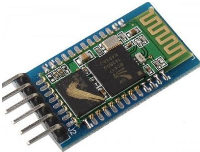
FIGURE 3.4B: HC-05 (BLUETOOTH MODULE)
