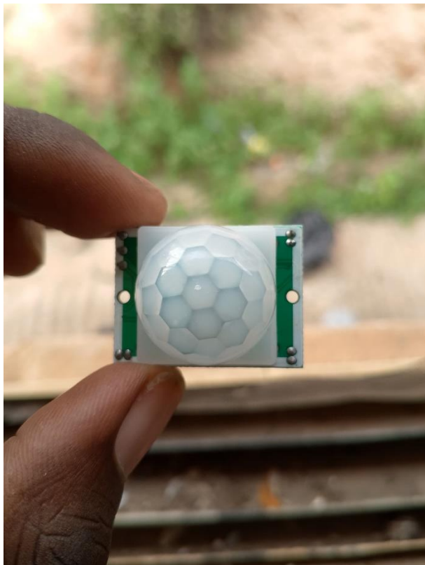
FIGURES 4.4B: LAYOUT OF THE MOTION SENSOR
