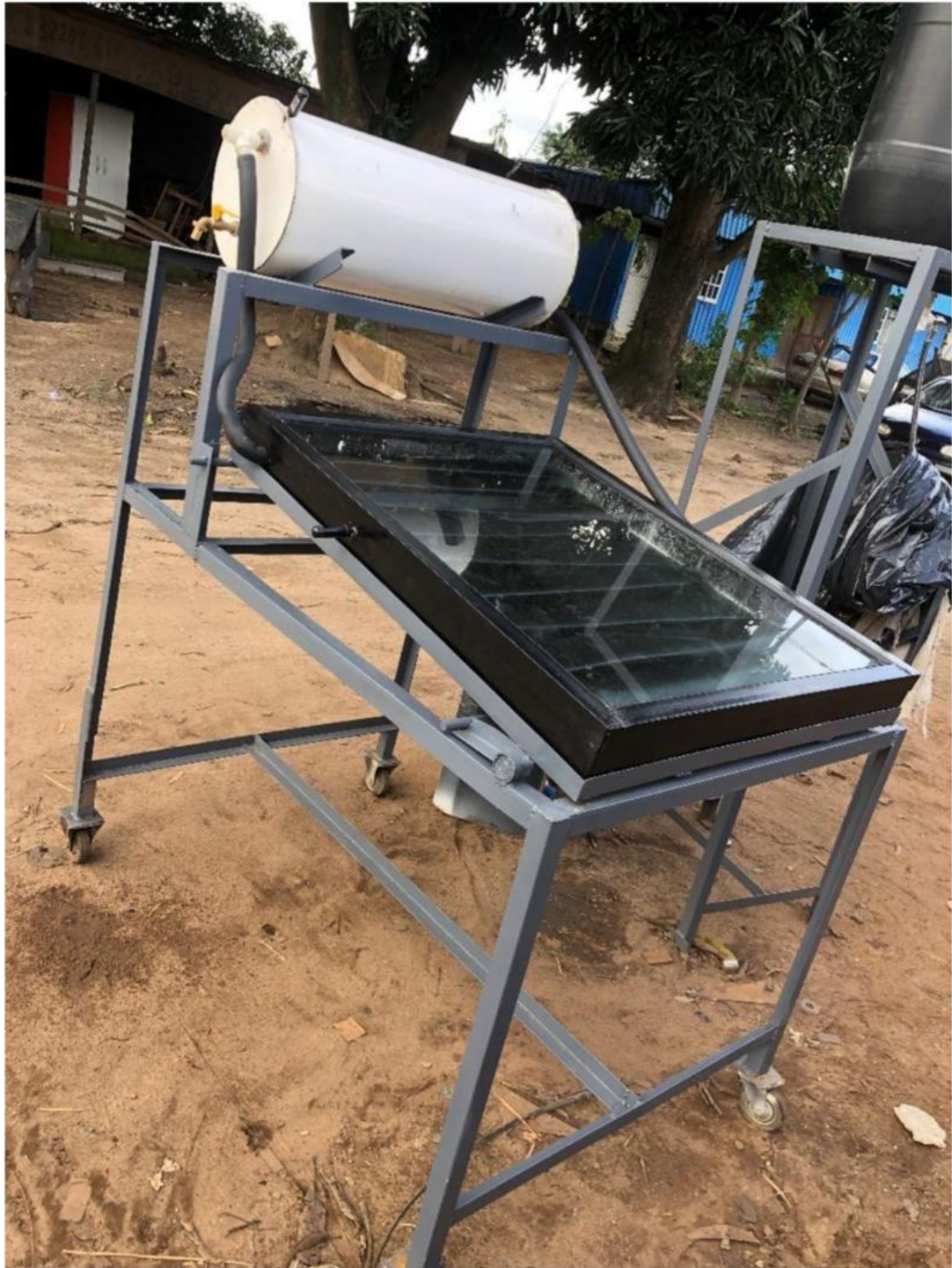
Fig 2.1 Domestic Solar heater using a Fresnel flat plate reflector
