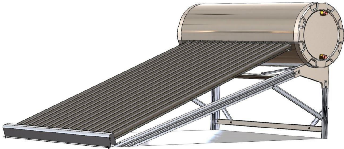
Fig 2.4 CAD DESIGN OF A SOLAR WATER HEATER USING SOLIDWORKS
