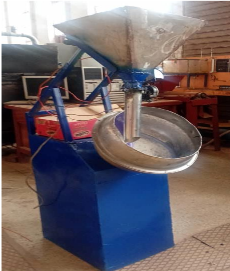
Figure 4.2: A Pictorial View of The Peanut Coating Machine
