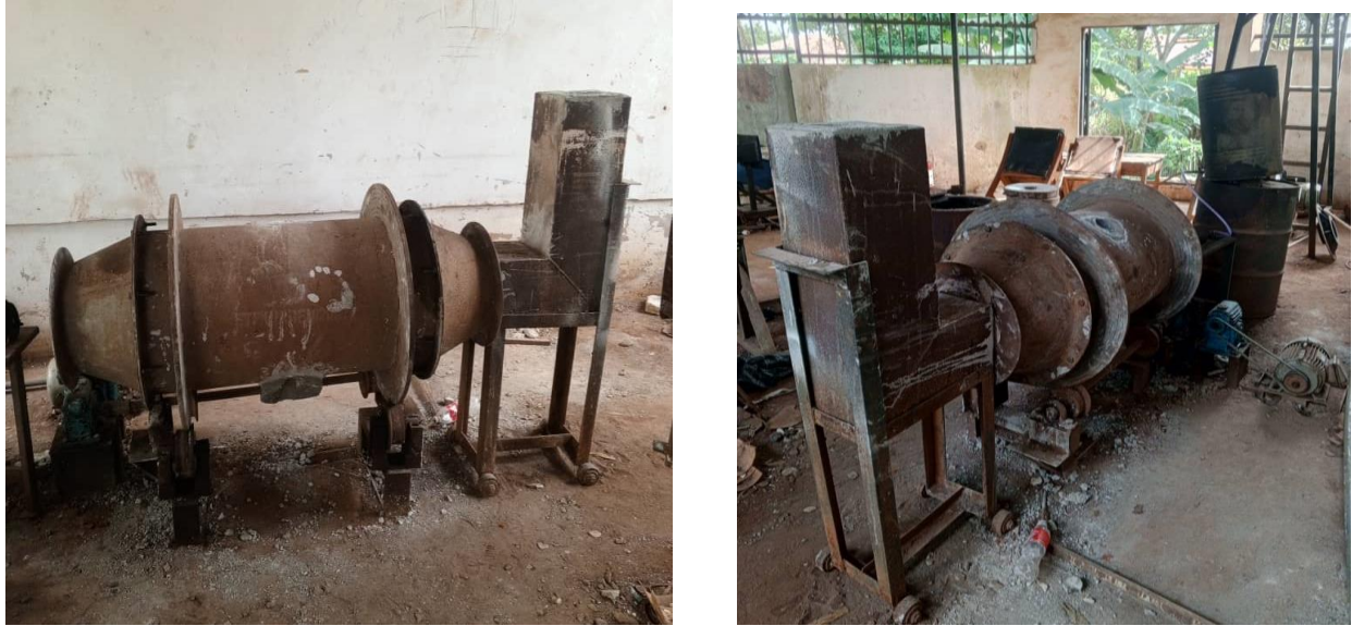
Figure 4.4: Structural body and shell
