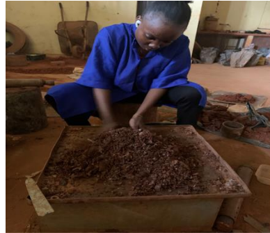
Carrying out compaction test
