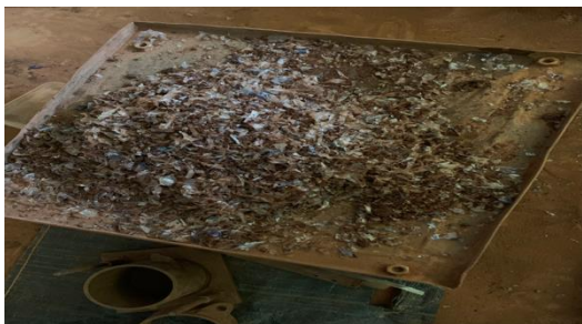
Soil and SPWS mix and compaction apparatus
