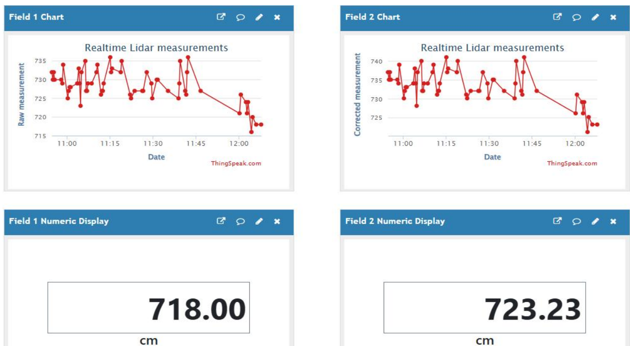
Plate 4.3: Screenshot of measurement chart and numeric display on Thingspeak dashboard
