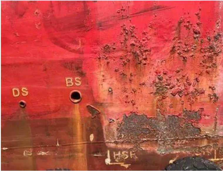
Figure 2.1: Uniform Corrosion on Ship a Hull
