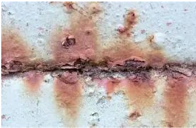
Figure 2.3: Crevice Corrosion on a Ship Hull
