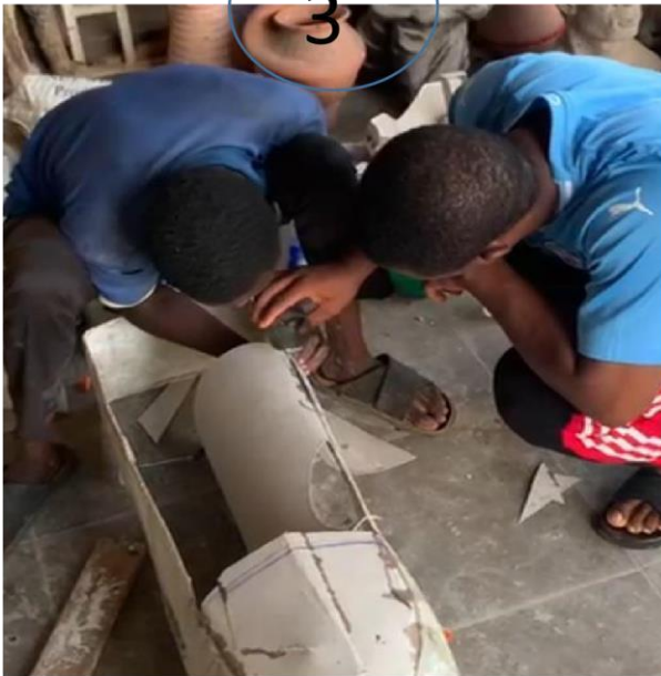
Getting the hull of ship from mold using Resin Catalyst and Fiber Mat
