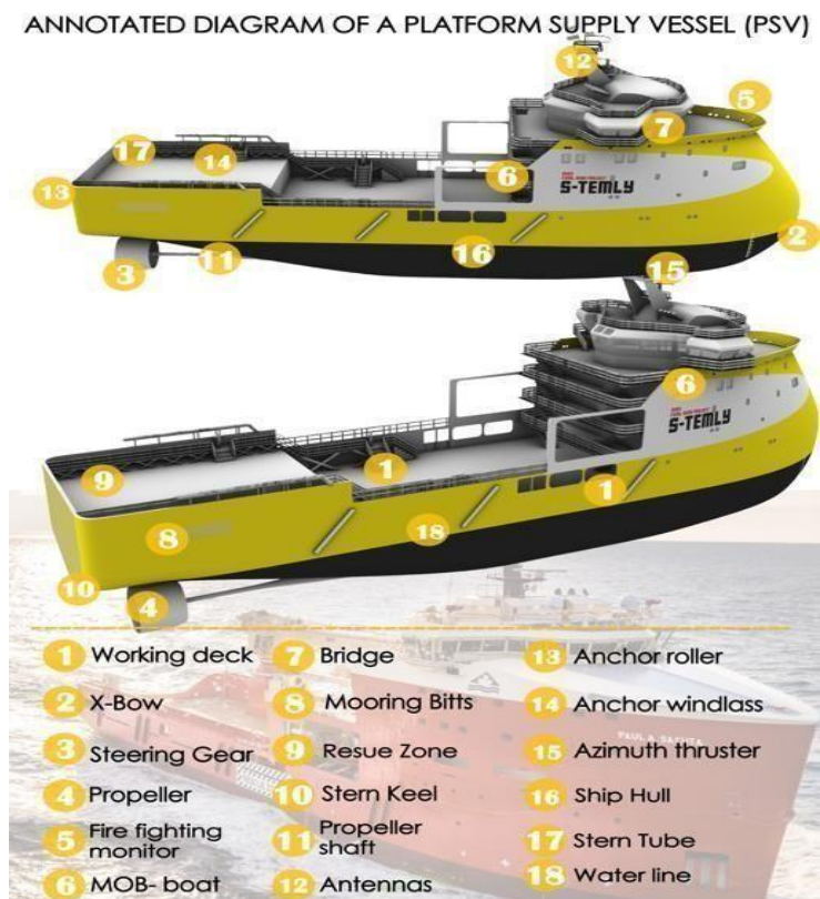
Fig 1. Annotated Diagram of ship vessel
