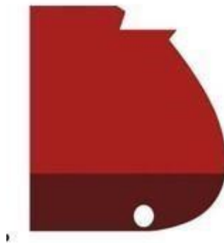
Fig: X-BOW typical sideprofile
