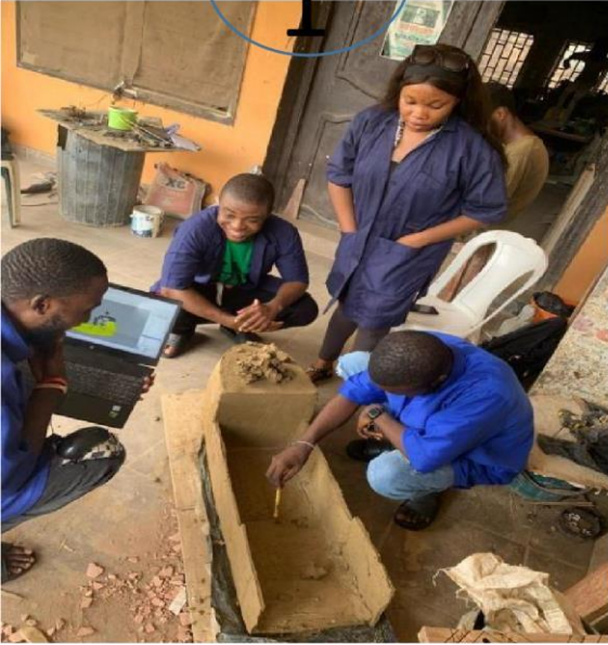
Getting Mold of Ship Hull using Clay
