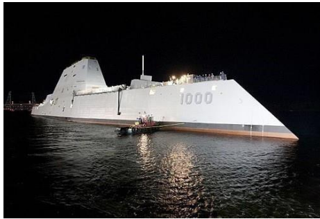
Fig: I; Zumwalt class destroyer with inverted bow inverted bow
