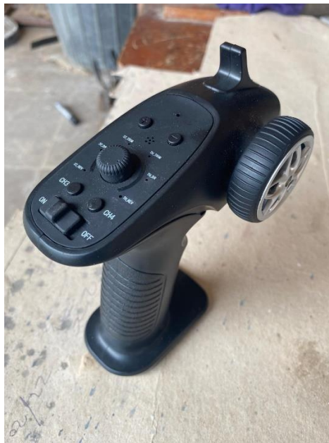
Fig 3.8: 2.4Ghz 4CH Radio Transmitter
