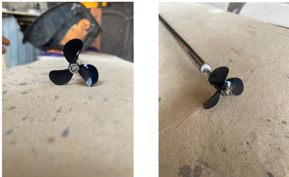
Fig 3.2 Plastic propeller with 30cm shaft.
