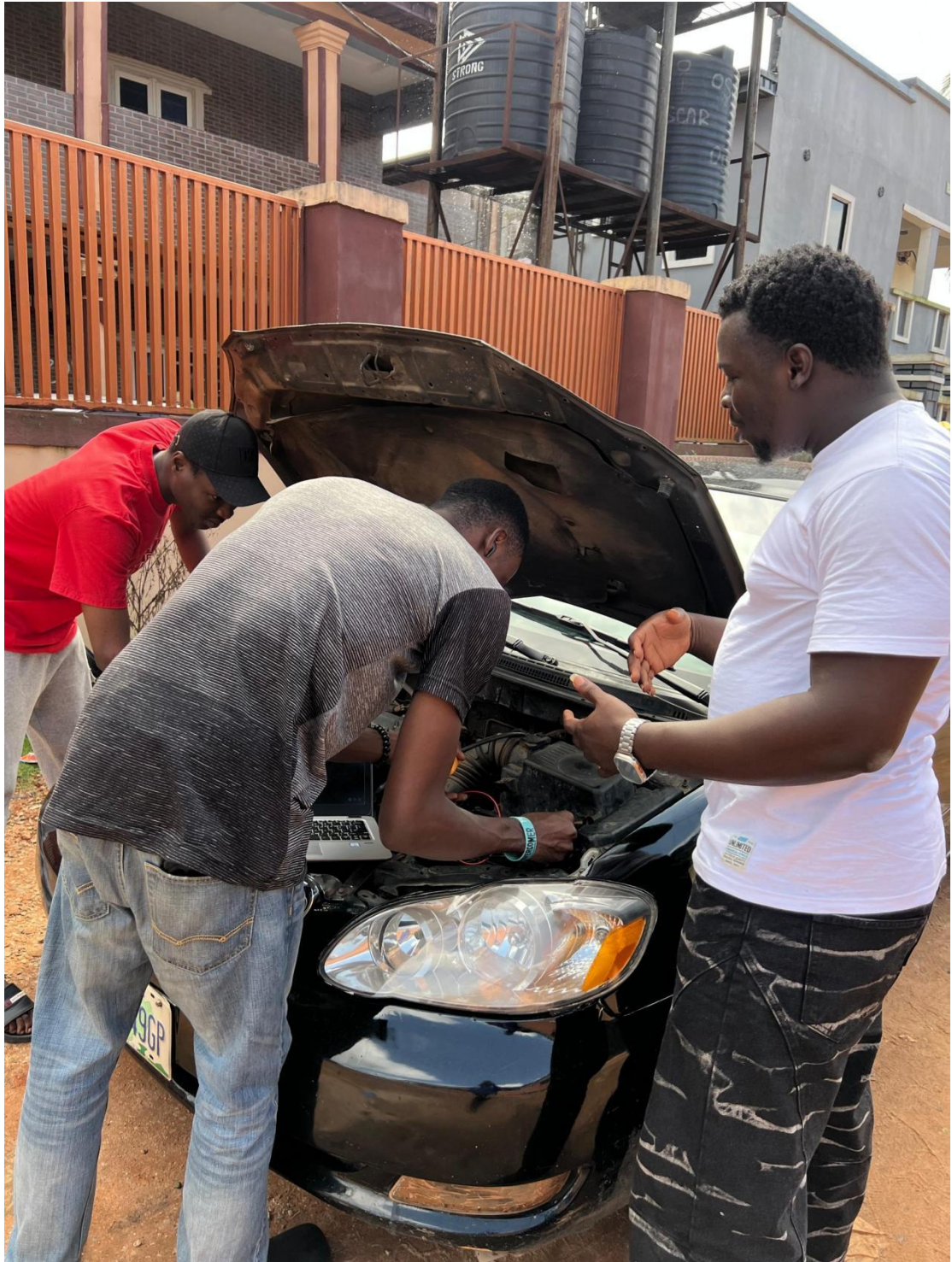
Fig 2.3 Checking Car Battery voltage.
