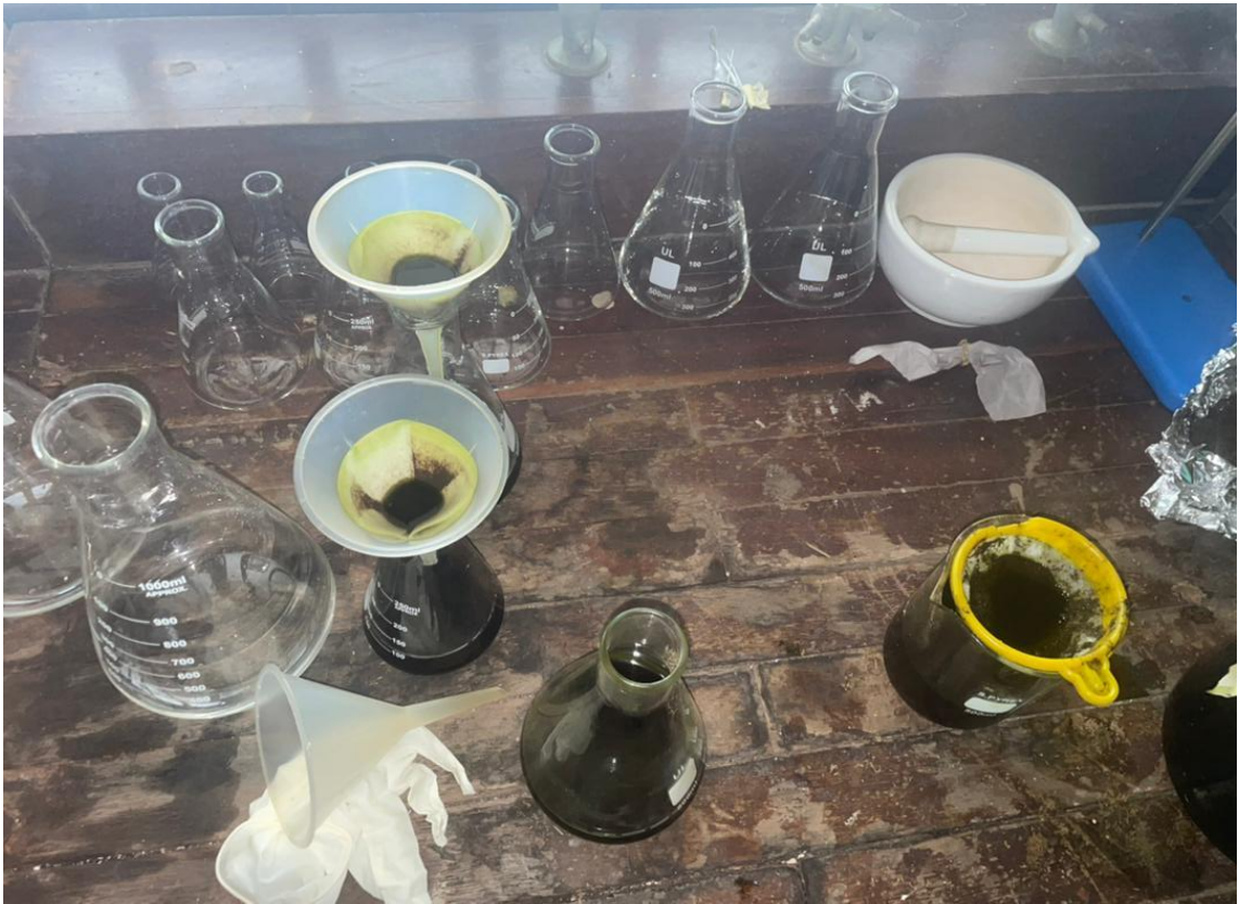
Filtration using Grade 1 whatmann filter paper
