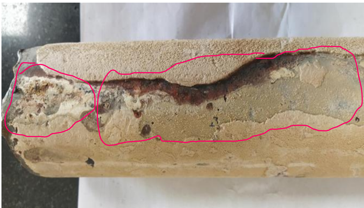
Figure 4.5: Layered deposits observed on the boiler tube surface.
