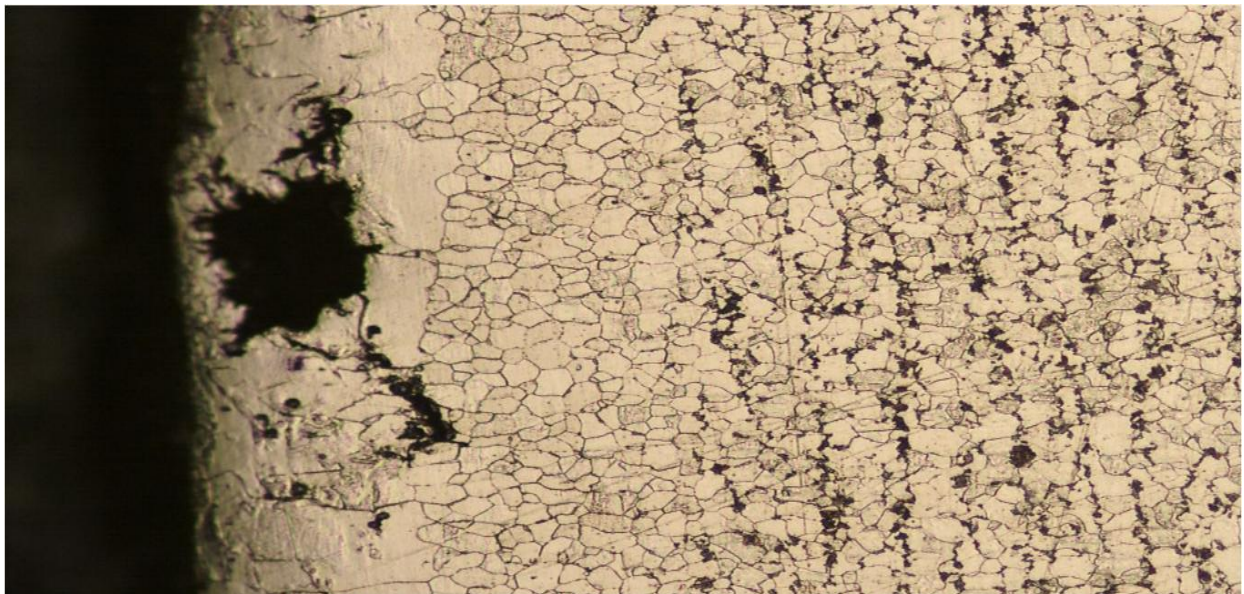
Figure 4.11: Evidence of thermal oxidation on the tube ID.
