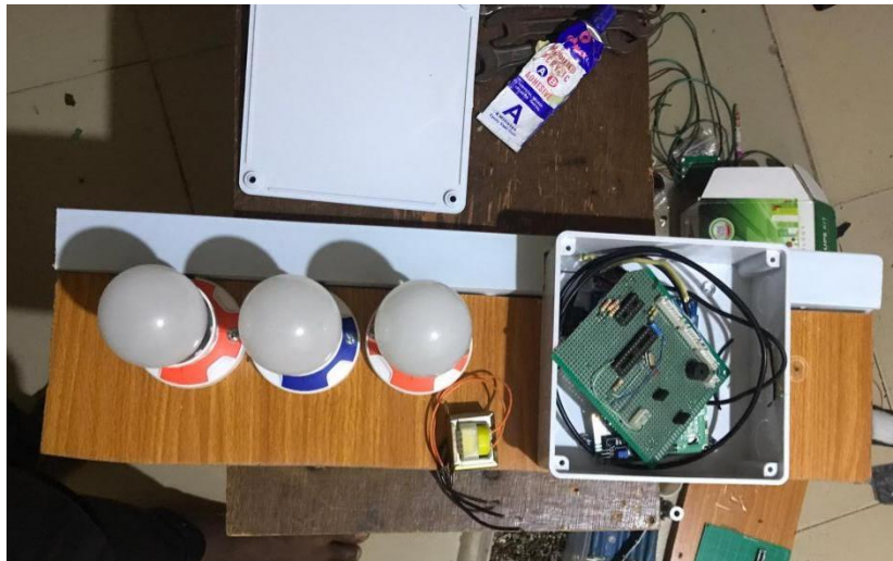
Figure 4.3 Three-Phase Induction Motor Protection System Prototype
