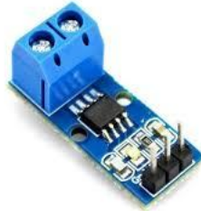
Figure 3.7 ACS712 Current Sensor
