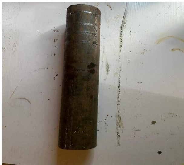
figure 3.15 The Non Corroded low Carbon Steel Pipe
