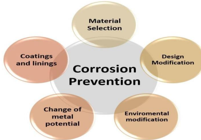
figure 2.12 Corrosion prevention methods (Smith J., 2021)
