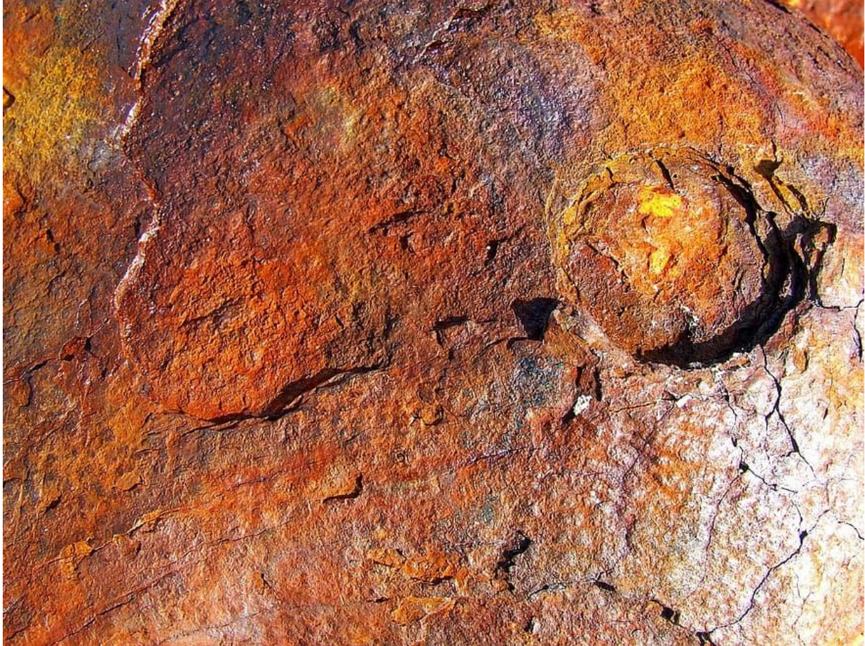
figure 2.5 The Schematic of General Corrosion of Carbon Steel in Aqueous Environment (Millenium Alloys, 2009).
