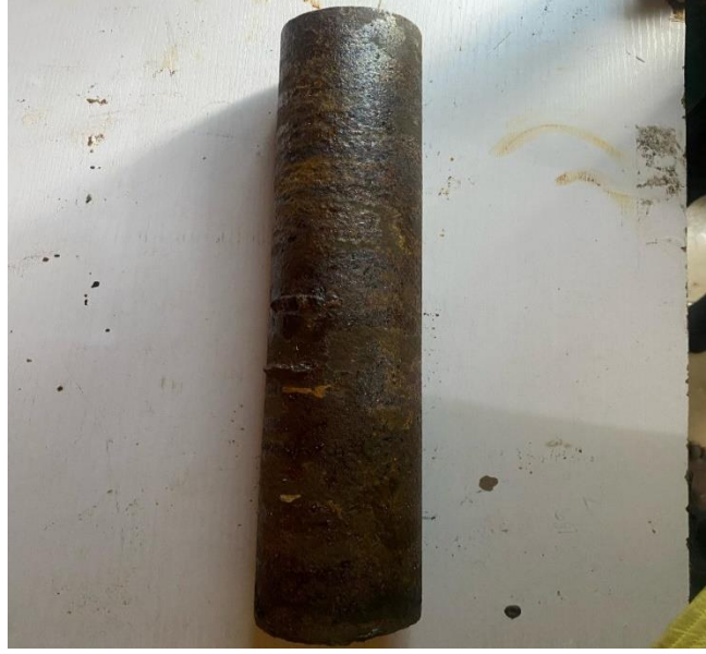
figure 3.16 The corroded low carbon steel pipe
