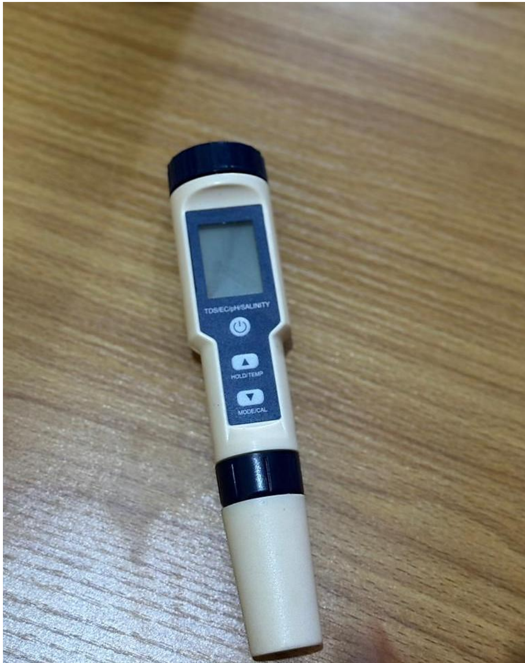
Plate 6: Multi-parameter (pH/TDS/Salinity/Conductivity/Temperature) meter
