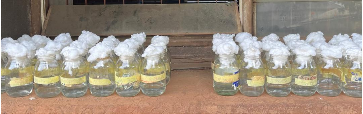
Plate 1: Culture vessels with varying concentrations of Hydrogen peroxide and microalgae Chlamydomonas (left) and Scenedesmus (right)
