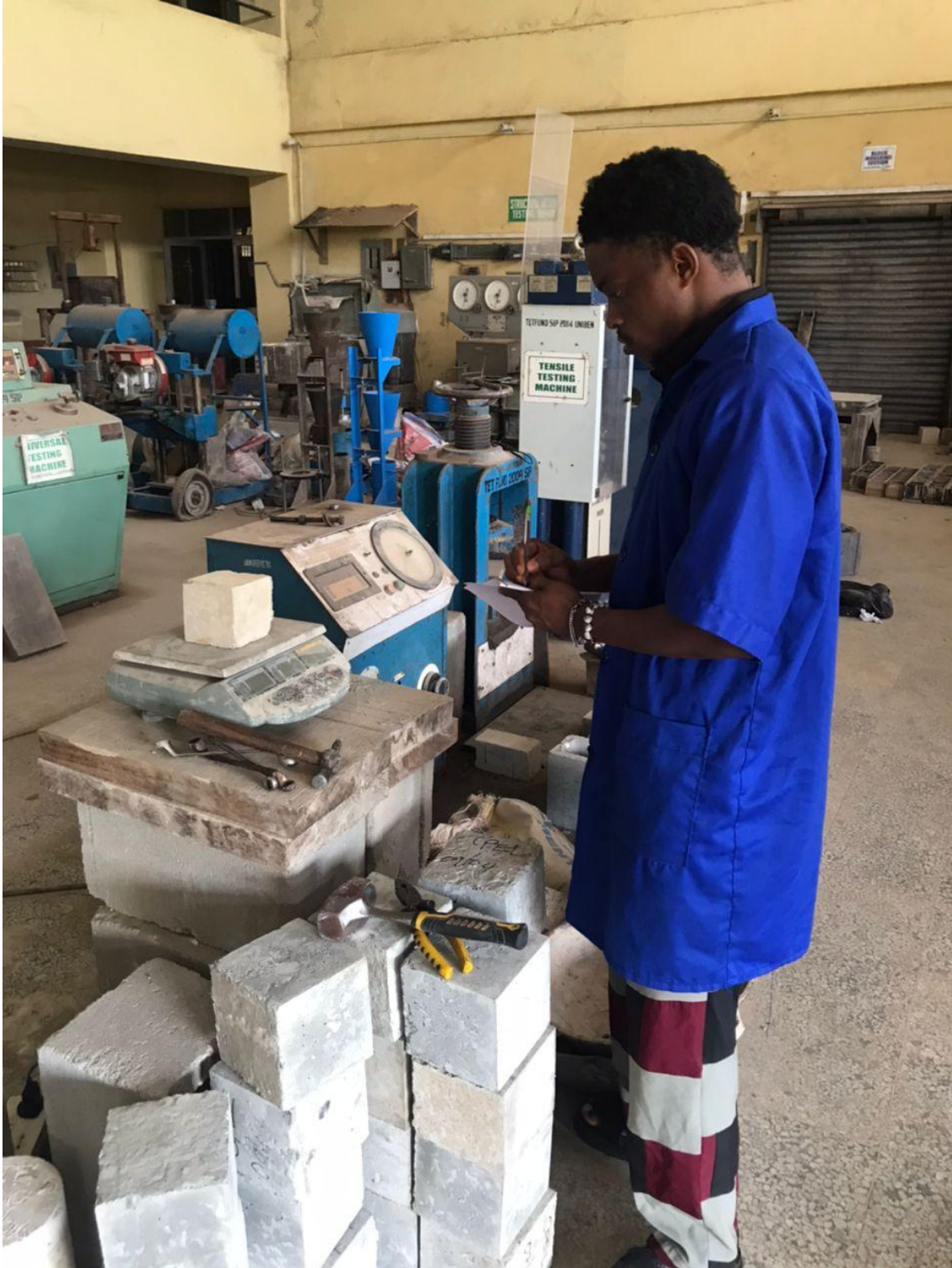
Plate 4: Concrete cube weighing
