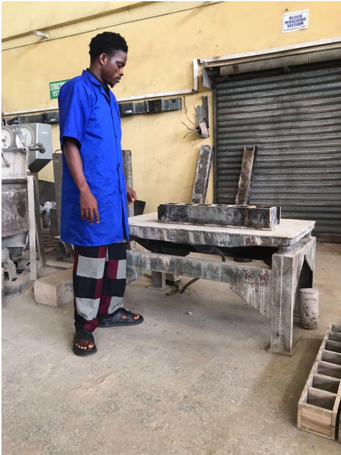
Plate 5: Concrete mix vibration
