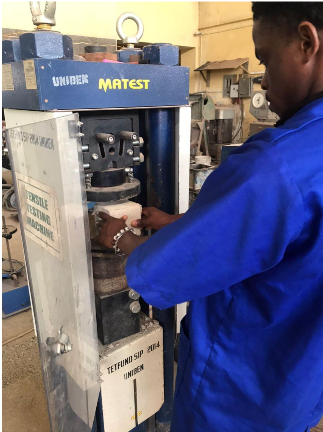
Plate 2: Compressive strength test in the lab
