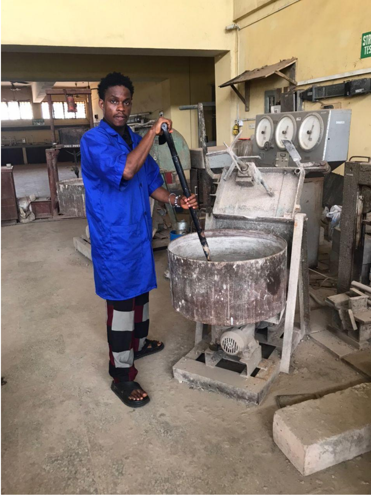
Plate 3: Concrete mixing with partial ceramic tile replacement
