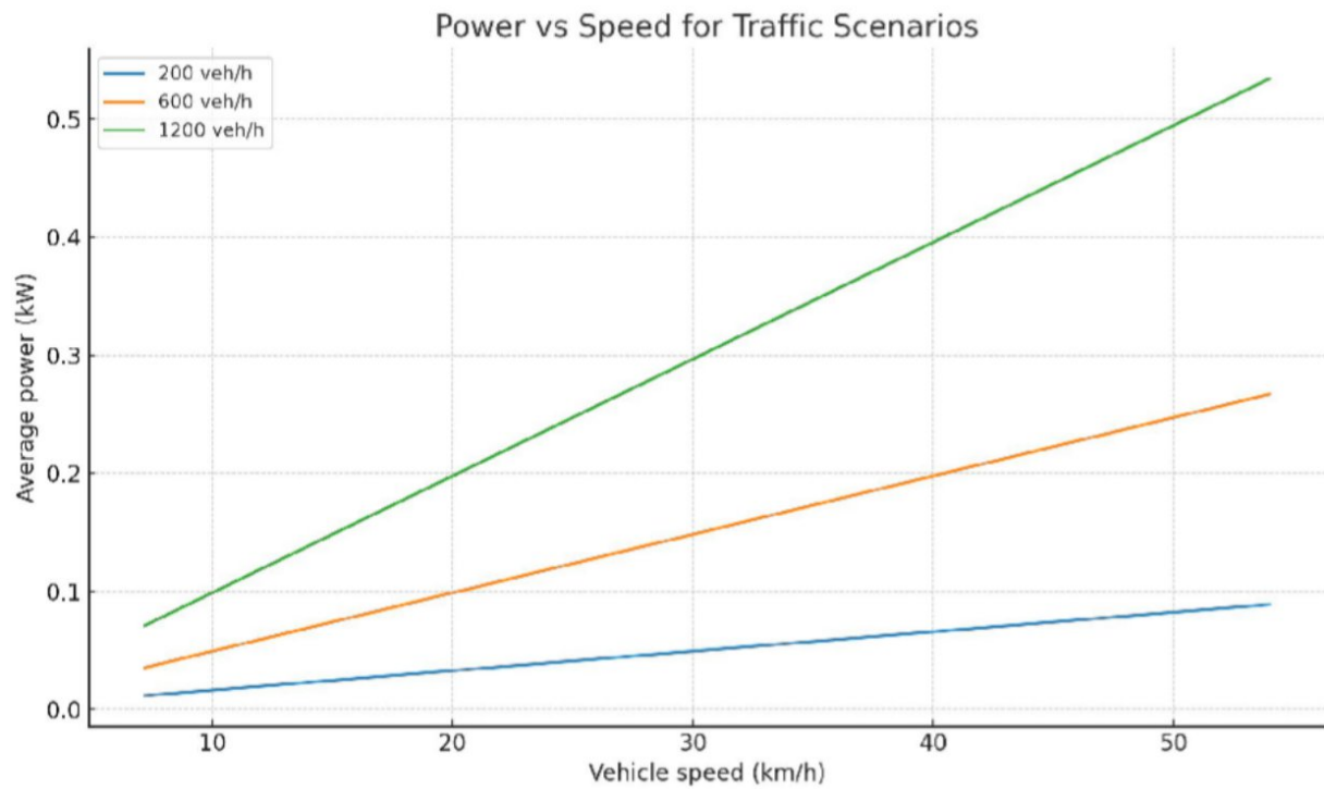
FIGURE 4.1: Shows Power Vs Vehicle Speed For Different Traffic Scenarios.
