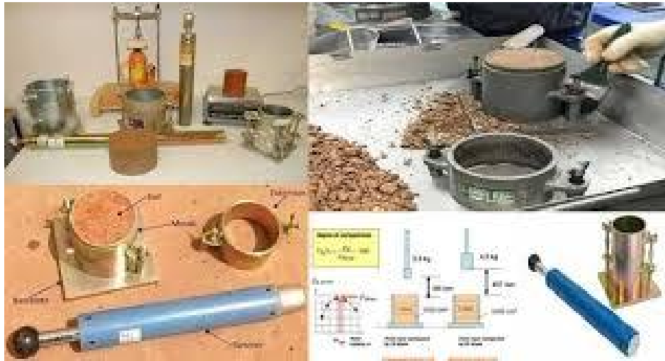
Fig 3.3 Soil Compaction test ( Mishra, 2015)
