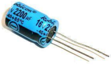
Figure 2.4: Capacitor (Build Electronic Circuits, 2014)
