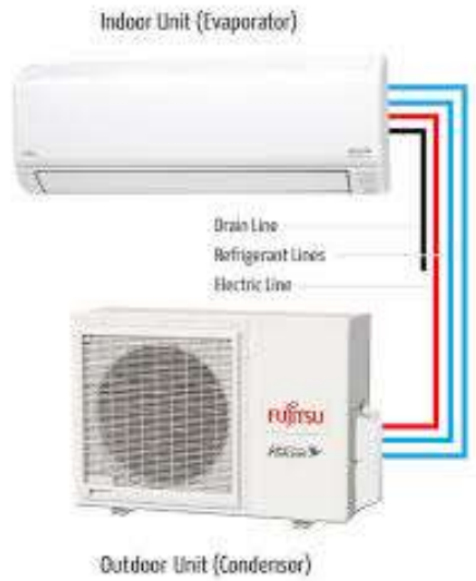
Fig 2.4 Ductless mini-split systems
