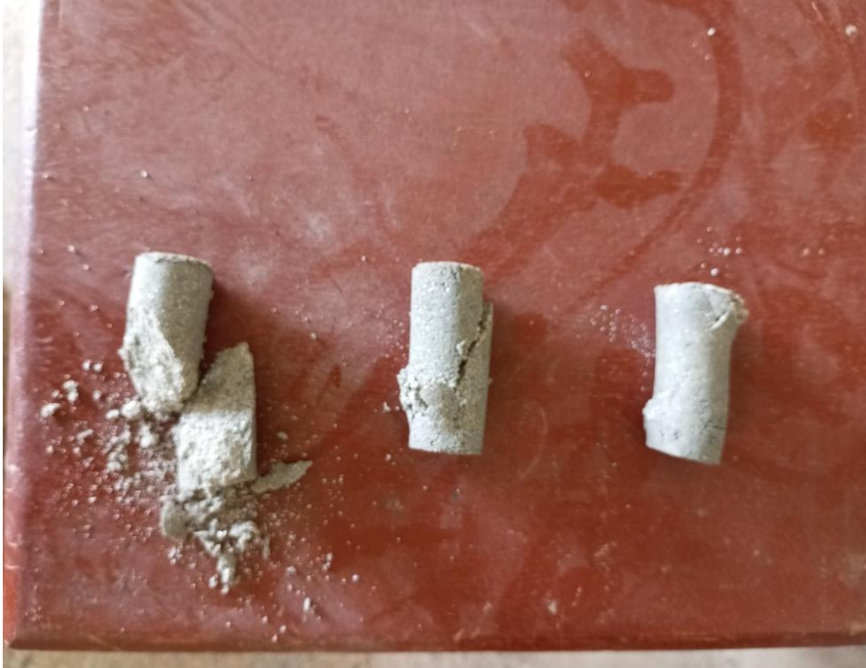
Figure 4.3.3 Image of the composite materials of all ratios after going through tensile test
