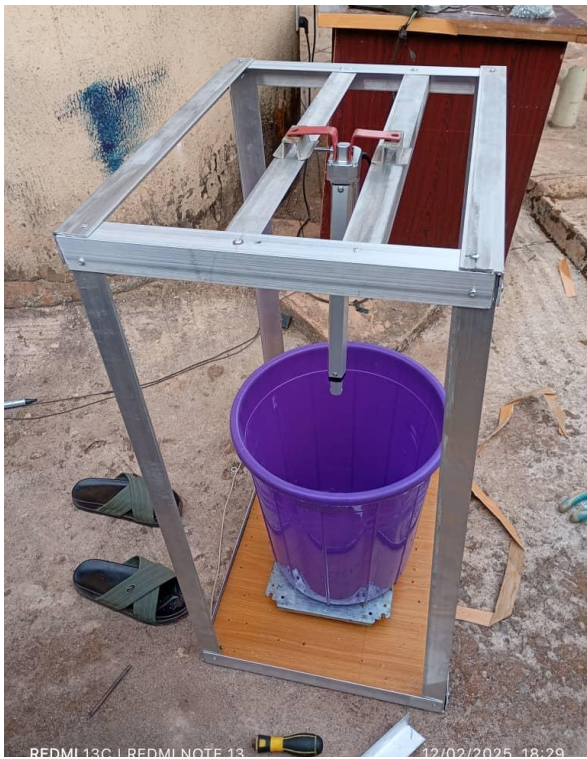
Fig. 3.14: Mounting up the Actuator on the Frame for Compaction
