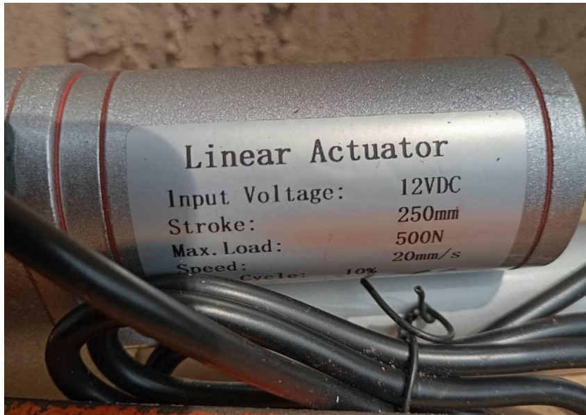
Fig. 3.15: Linear Actuator for Compaction
