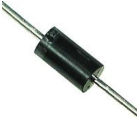
Figure 11: A 1N4148 Diode
