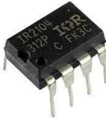
Figure 4: IR2104 MOSFET Driver
