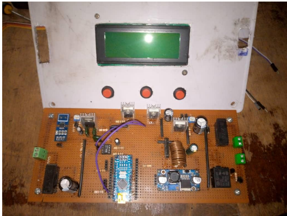
Figure 19: Solar Charge Controller on the Veroboard
