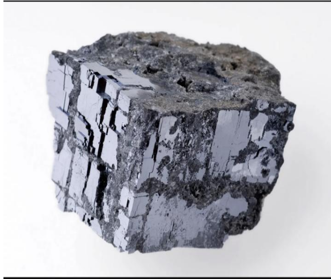
Fig 2: Galena (lead sulfide) sample. From lead; Definition, uses, properties and facts, Encyclopaedia Britannica. (2025,september 24).
