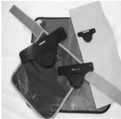
Figure 2.4: Gonad shields with sheet of lead rubber for gonad protection.
