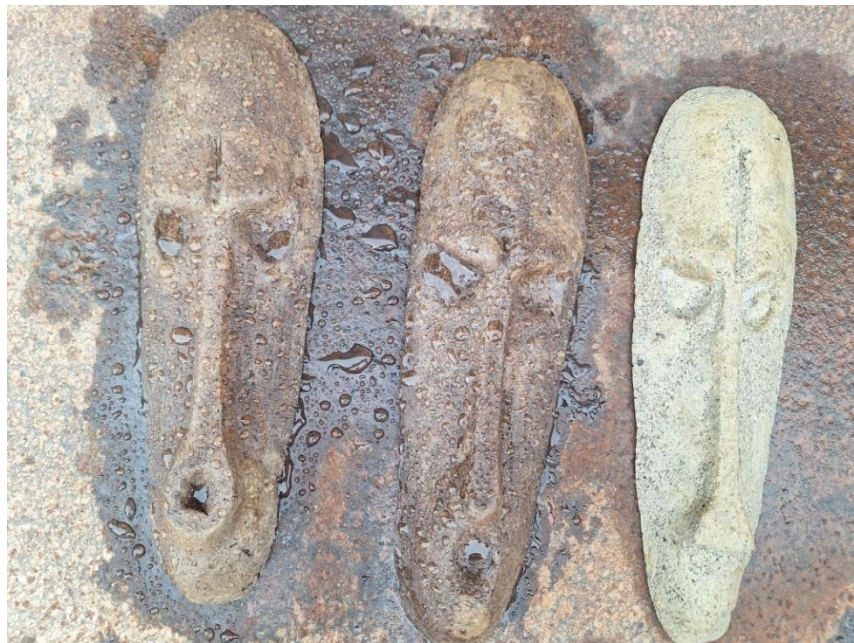
Pilot Study Observing Waxed Polystyrene Samples after the Rain. Photographed by John Anabui Year: 2025
