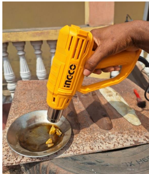
Pilot Study of Heat Gun melting wax Photographed by John Anabui Year: 2025
