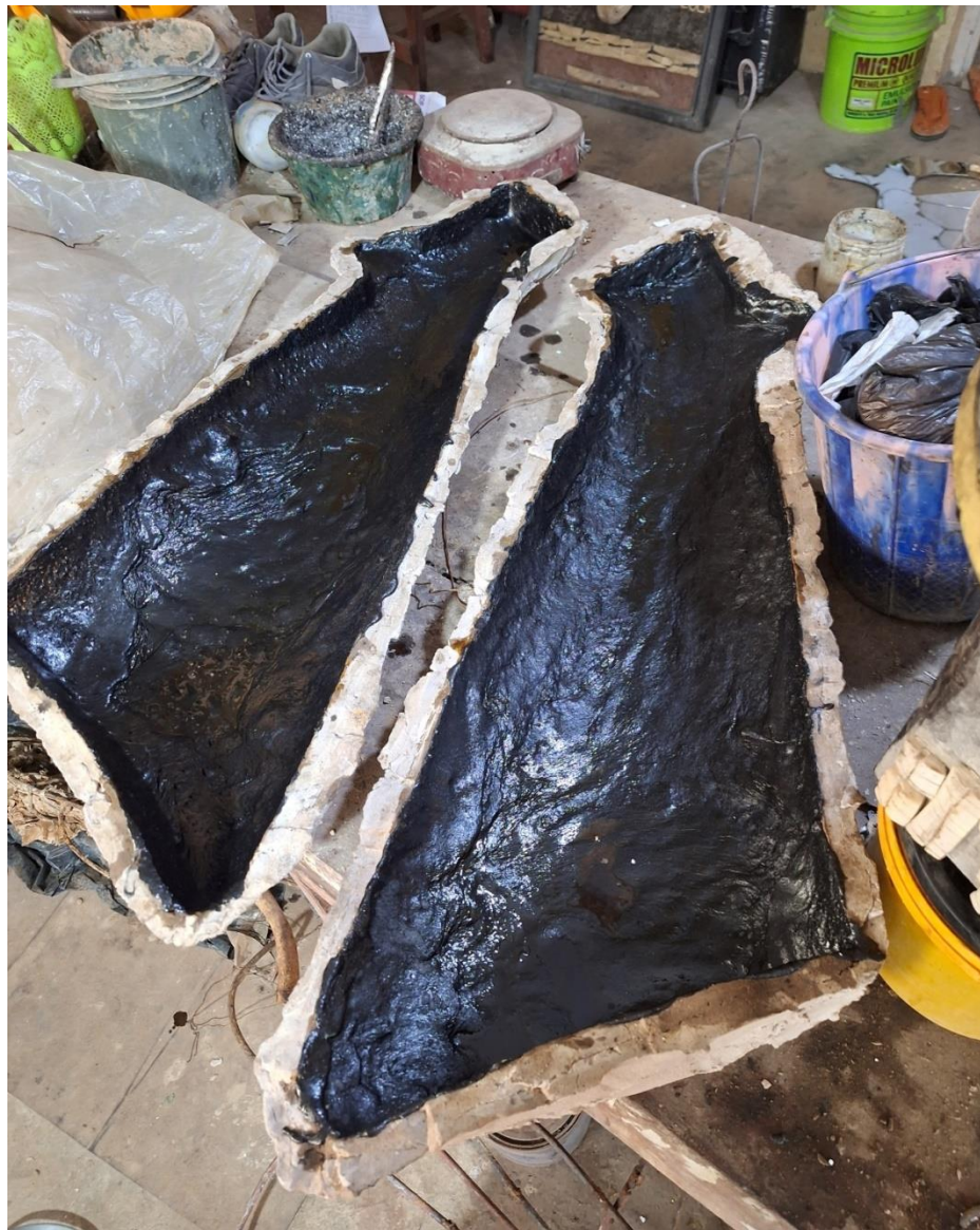
Cast of the buttstock Photographed by John Anabui Year: 2025
