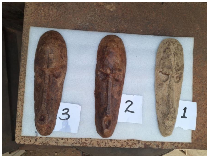
Pilot Study Samples of Wax Polystyrene for Weather Testing. Photographed by John Anabui Year: 2025
