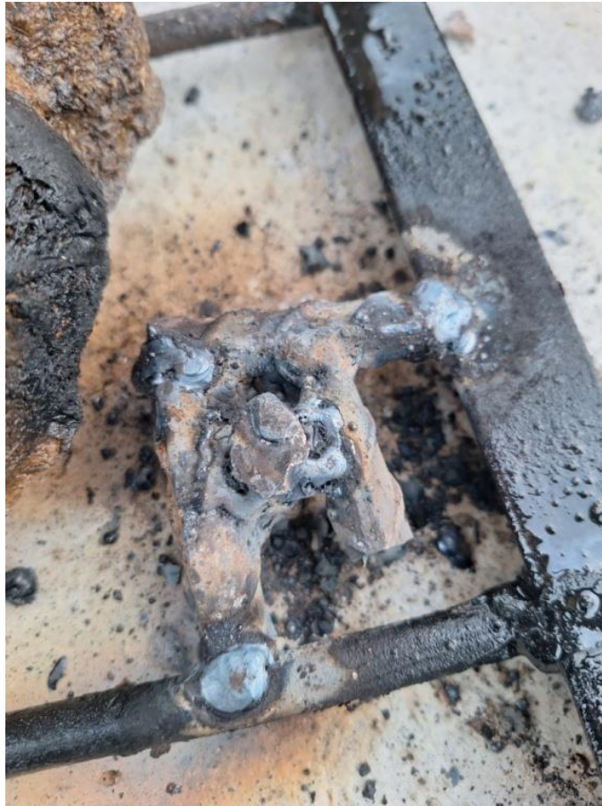
Welding of the sculpture's base to the top of the plinth Photographed by John Anabui Year: 2025
