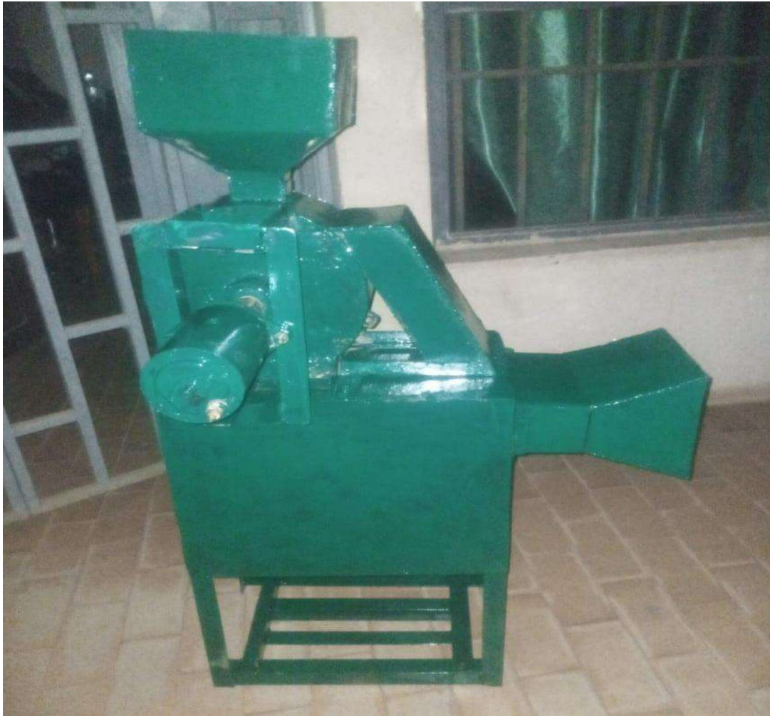
Fig.4.1 Final assembly of the DC powered melon sheller
