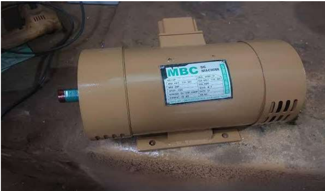
Fig 3.10 1 horsepower (HP) DC Motor
