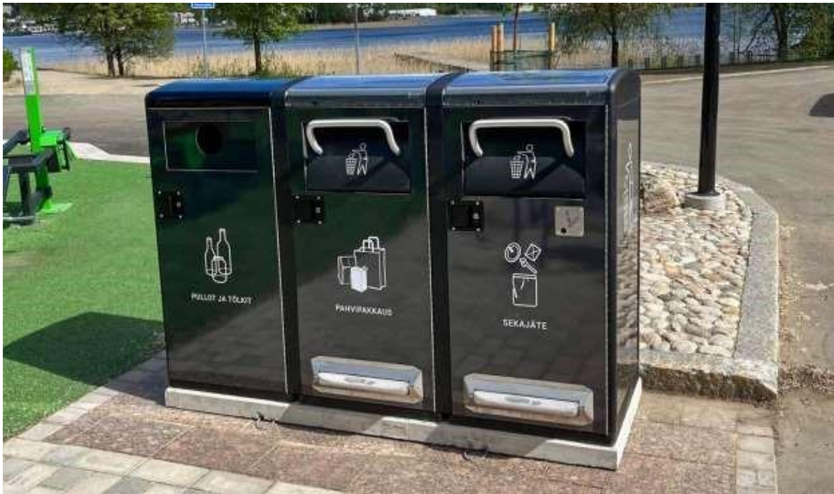
Figure 2.3: Internet of Things (IoT)-Enabled Smart Waste Bins
