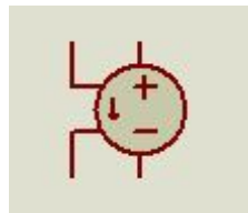
Figure 3.7: Current Controlled Voltage Source
