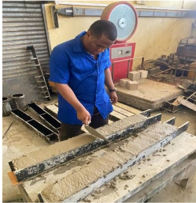
Figure 3.1: Casting of Cubes
