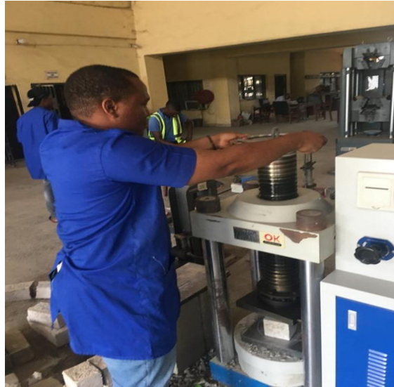
Figure 3.2: Compression Test on Hardened Cube
