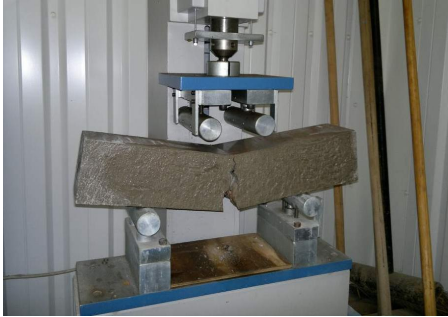
Plate 5: Crack pattern and Mode of failure of beam specimen
