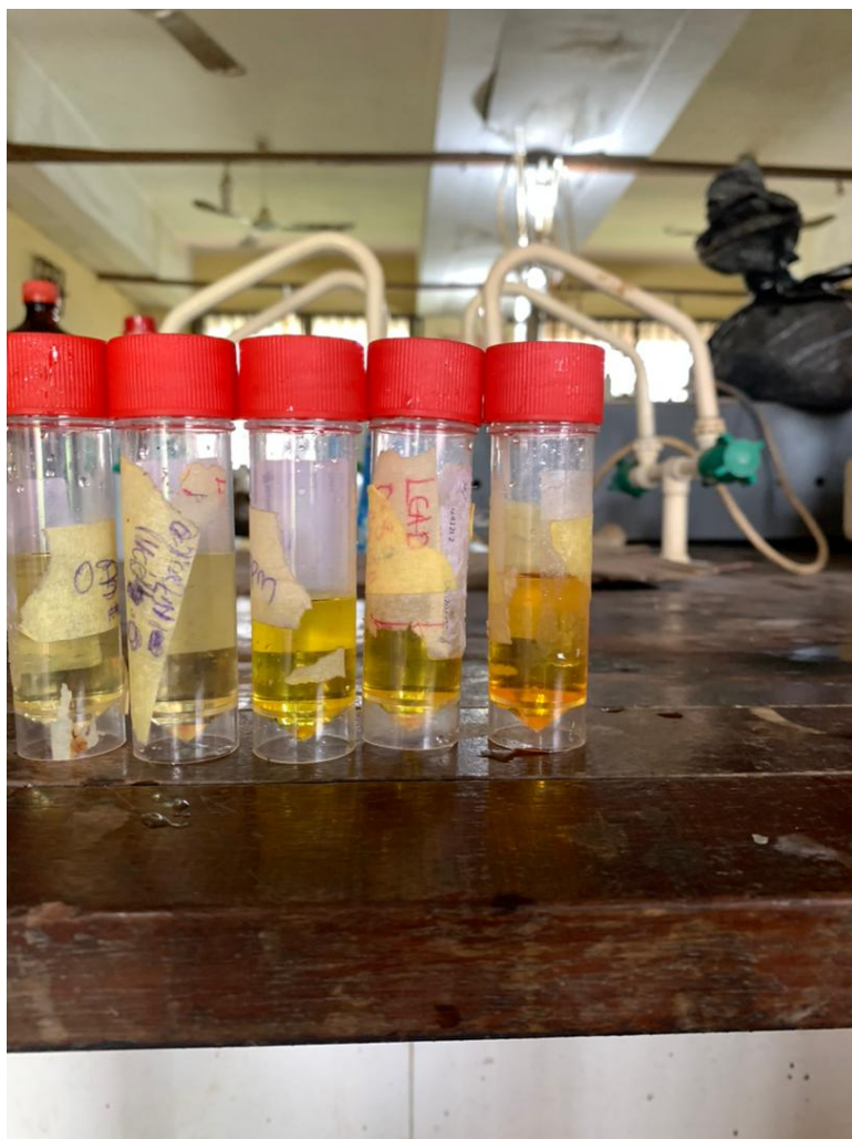
Figure 2.3: Prepared Nitrate Standards for calibration
