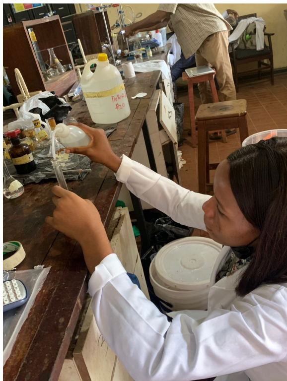
Figure 2.4: Preparation of sulphate standards for Calibration
