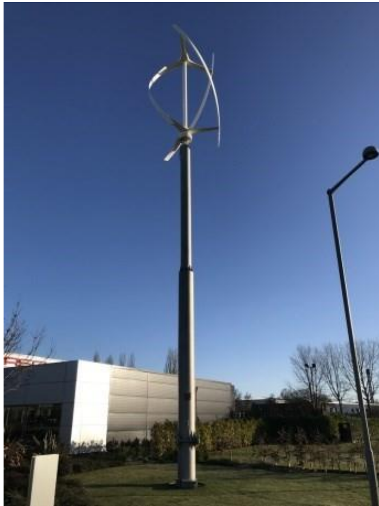
FIG 2.3: Helical Savonius Vertical Axis Wind Turbine.
