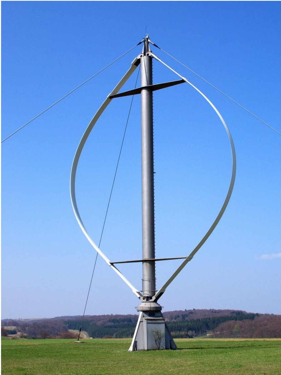
FIG 2.4: Darrieus Vertical Axis Wind Turbine
