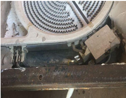
Figure 26 Heat Resistant Conductor for Internal Wiring
