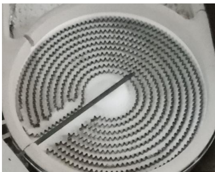
Figure 23 The Heat Generating Compartment
