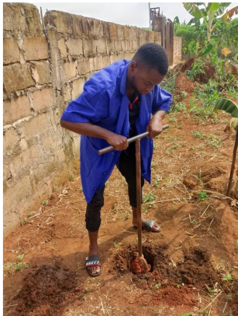
Plate B - 4 Extracting of soil sample with an auger
