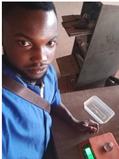
Plate B - 2 Weighing the density bottle with water filled to the brim
