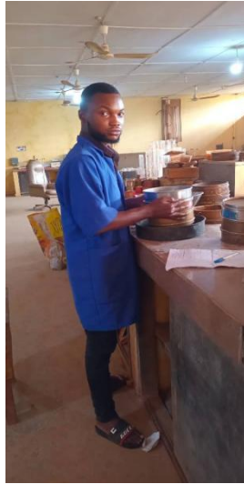
Plate B - 1 Sieving the soil sample
