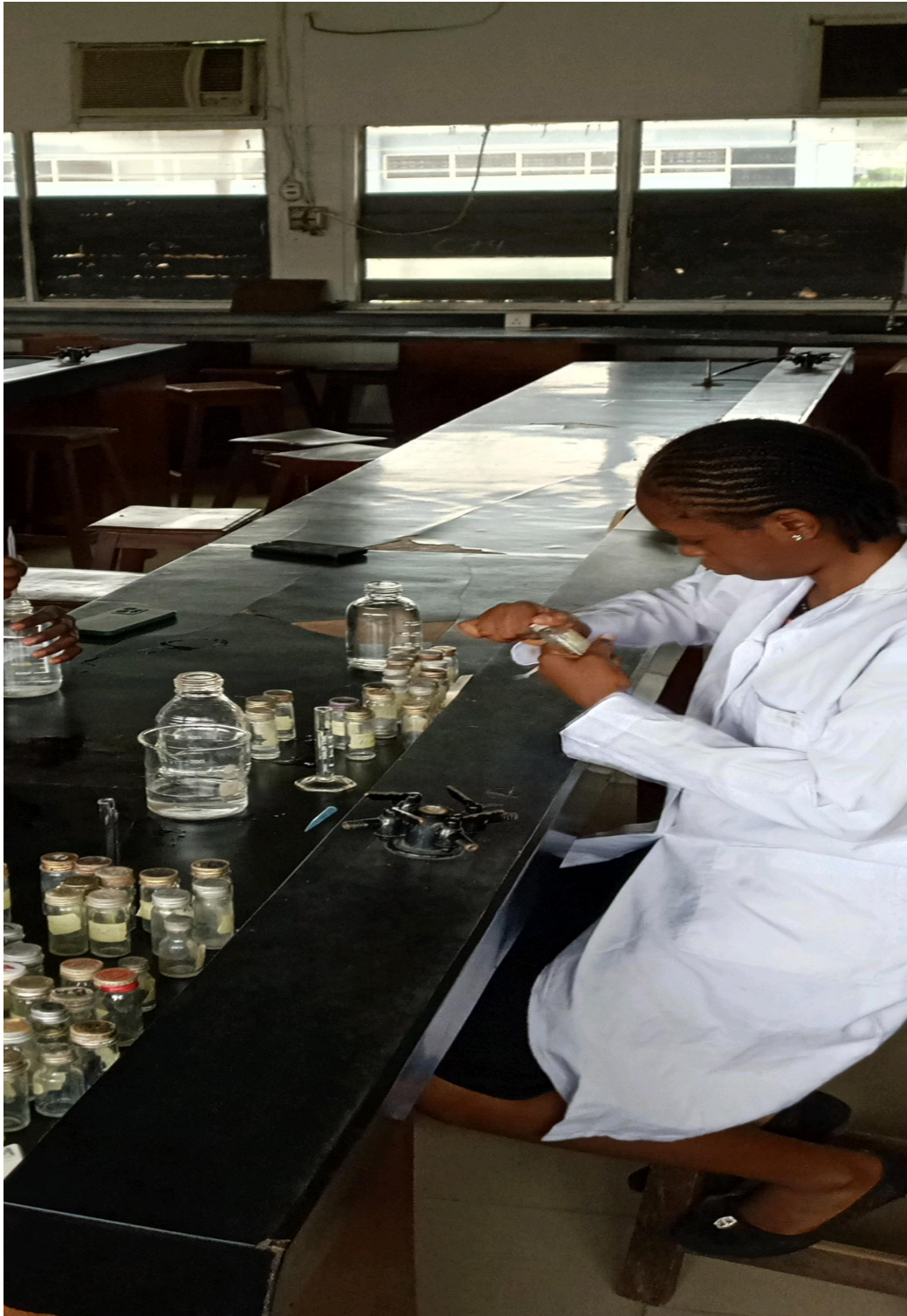
Picture showing preparation of Quarter - Strength Ringer's solution and dispensed into sterile bijou bottles.
