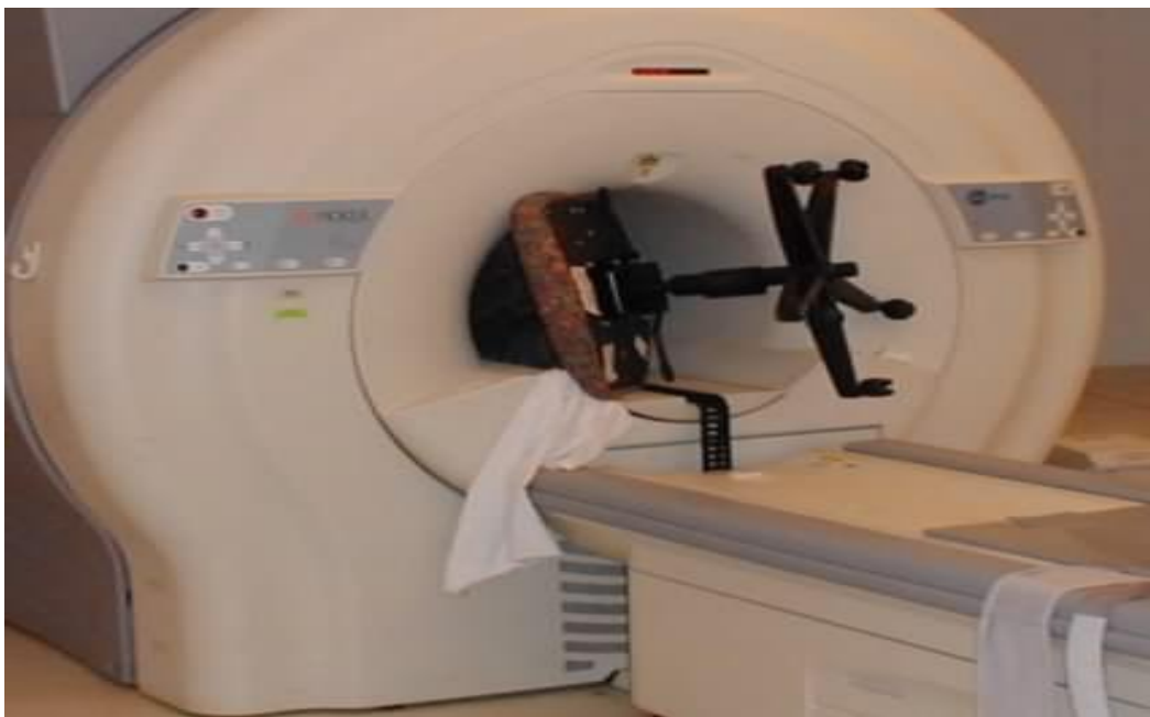
Fig. 3_ displays a metal chair inside the MRI scanner, which is another example of a projectile hazard. (UCSF Radiology et al., 2015)
