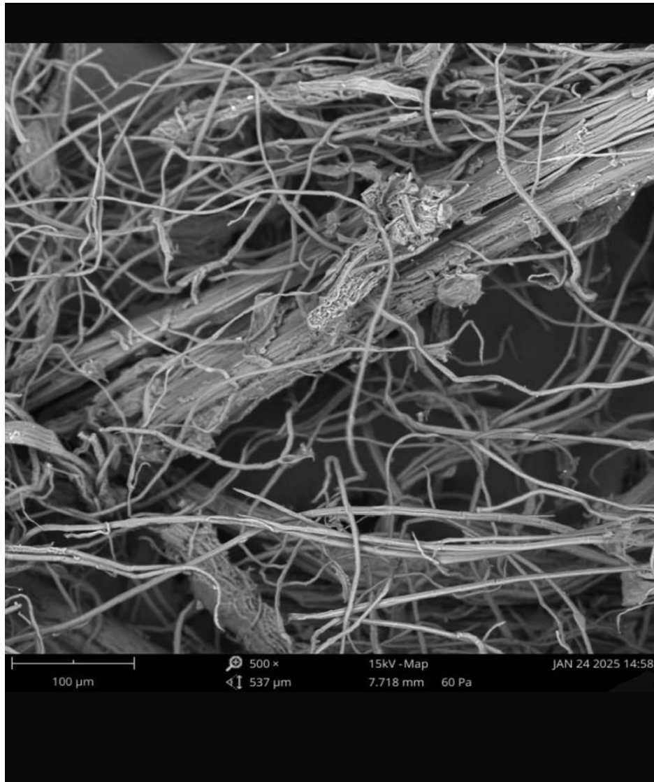
Figure 3.3: SEM image of the sample of cellulose extracted from rattail grass at magnification 500
