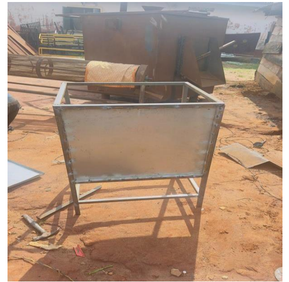
Plate 3.3: Assembly of oven chamber
