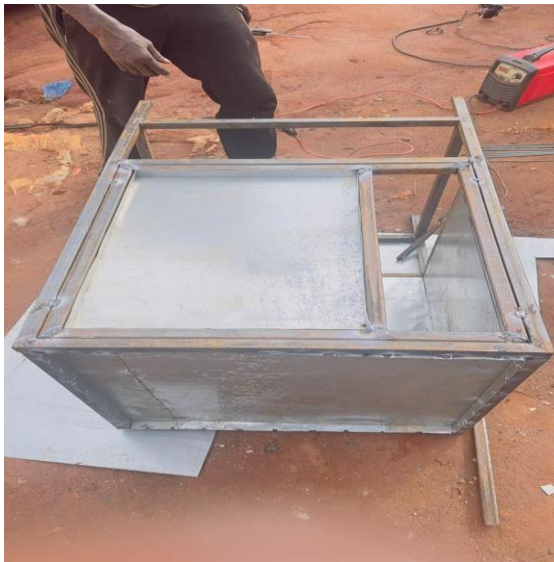
Plate 3.3: Assembly of oven chamber
