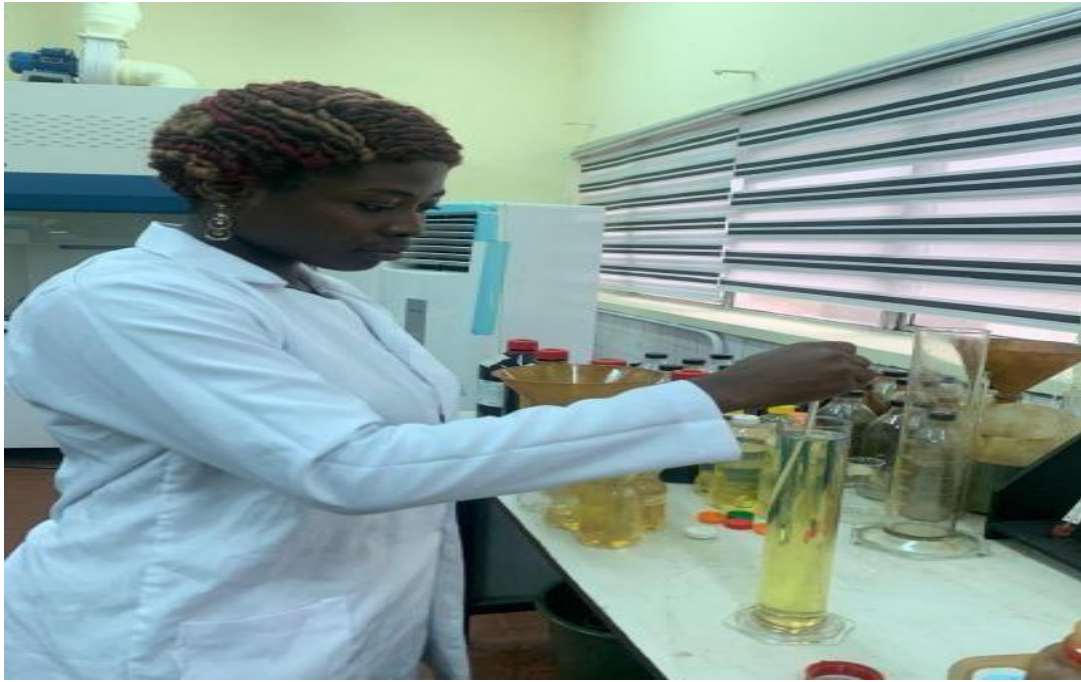
Figure 2.3: Set-up for Density determination using an hydrometer method
