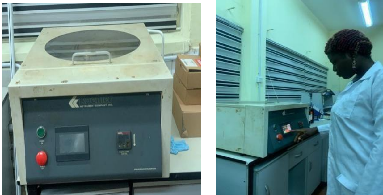
Figure 2.3: (a) koehler Laboratory Centrifuge for determination of BSW (b) a view of when I was carrying out the determination
