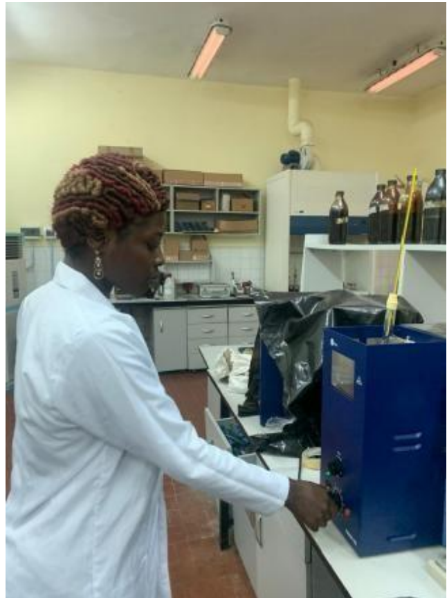
Figure 2.2: (a) Stanhope-seta Distillation unit for determination of distillation characteristics (b) a view of when I was carrying out the determination
