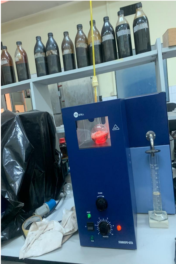
Figure 2.2: (a) Stanhope-seta Distillation unit for determination of distillation characteristics (b) a view of when I was carrying out the determination
