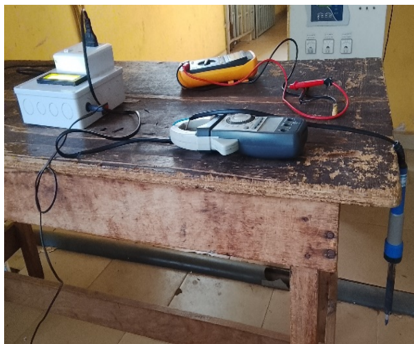
Fig 4.20: Actual data being measured and collected for 30W and 60W soldering iron.
