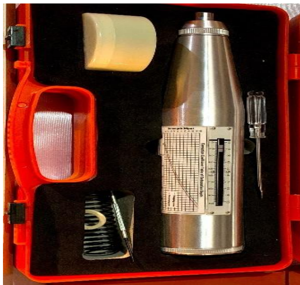
Figure 3.4: Schmidt rebound hammer used for surface hardness testing.
