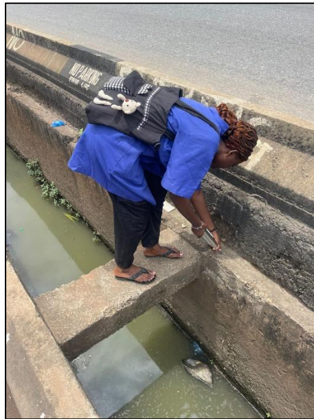
Plate A1: Field measurement of channel depth and siltation.
