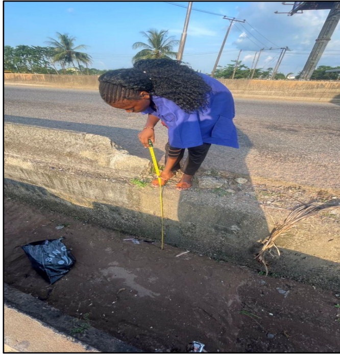
Plate A1: Field measurement of channel depth and siltation.
