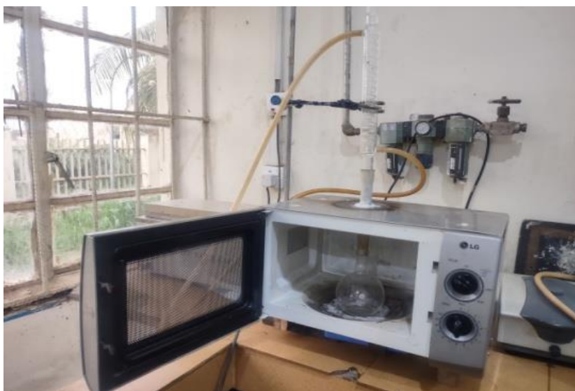
Plate 3. 1 Microwave aided biodiesel production setup
