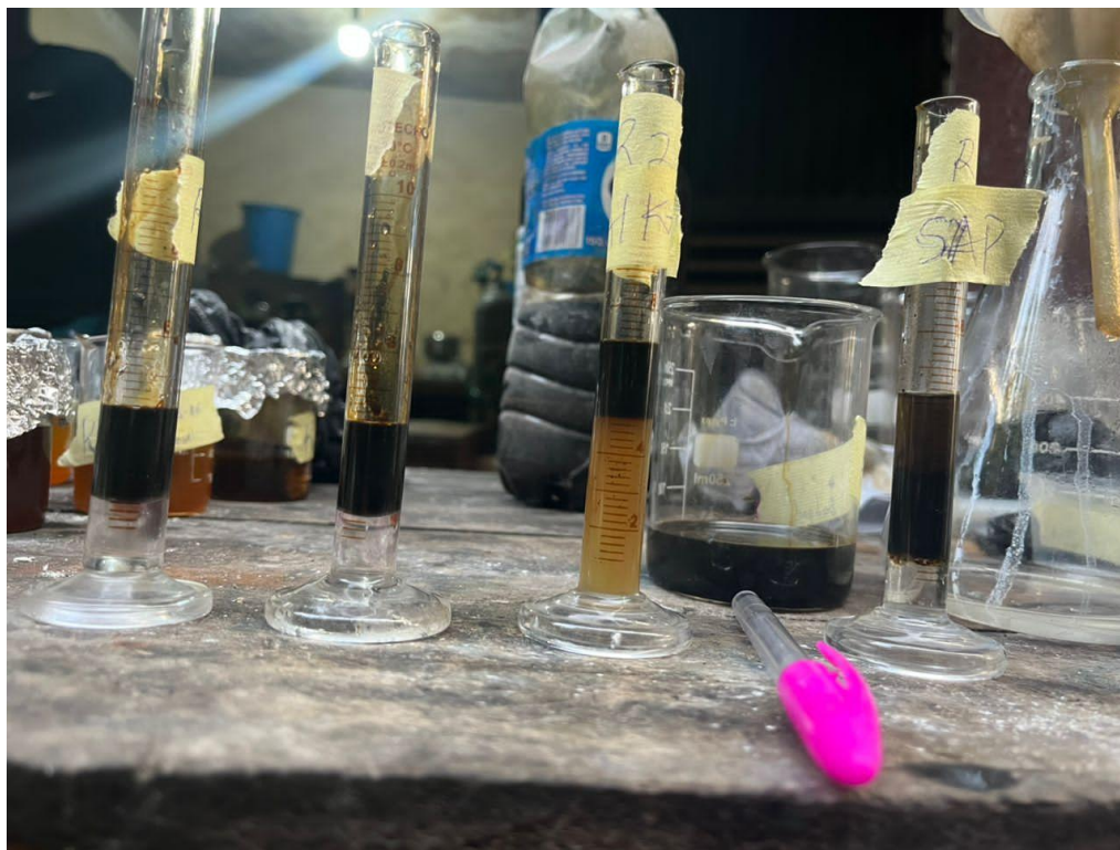
Plate3. 6; emulsification test of surfactant blend with crude oil and water and alkaline solution.
