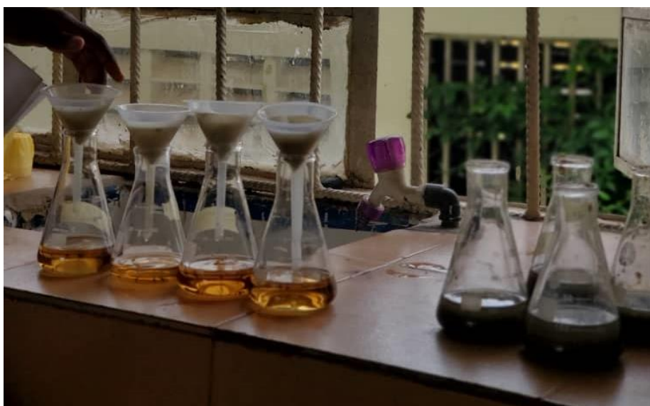
Plate 3. 3 filtration of the blended aloe vera and ethanol mixture
