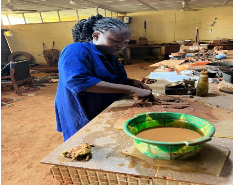
Plate C- 4: Researcher carrying out Atterberg limit test
