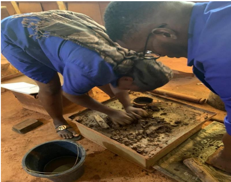
PlateC- 5: Researcher carrying out Compaction test
